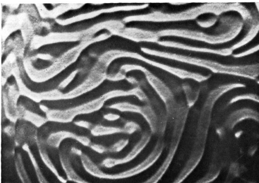
FIG. 1. Schlieren pattern in a 3-mm layer of carbon tetrachloride evaporating into still air, when the liquid surface has been contaminated with a trace amount of paraffin wax.
